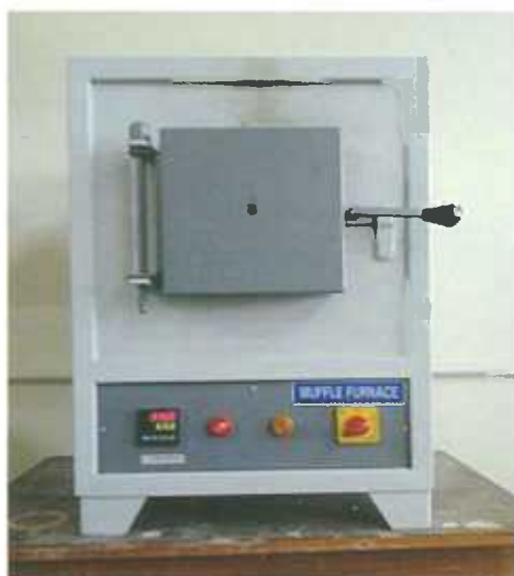
Figure 1: Muffle furnace with temperature option up to 1400 °C
